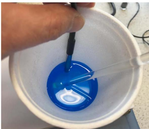
Avoid glass rod from contact with temp sensor
