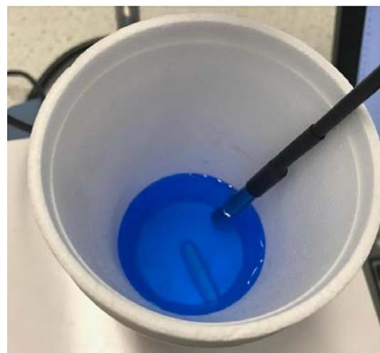
Magnetic Stir bar should not to contact with temp sensor
