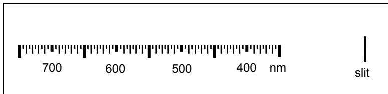
3. Take a piece of card and cut a hole ( $2\text{ cm} \times 2\text{ cm}$ ) at the centre of the card. Point the spectrometer slit (through the hole of the card) close to but not directly at the Sun. The card will shield your eyes from direct sunlight. You should see some dark lines called Fraunhofer lines after the discovery by Joseph Fraunhofer in 1814. Sketch these lines on the blank spectrum data sheet below.
