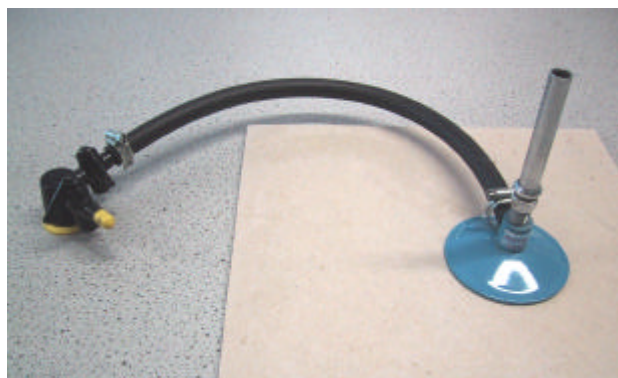
Both ends of rubber tubings should be held in position by hose clips
