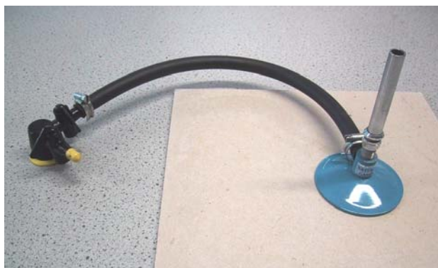
Both ends of a rubber tubing should be held in position by hose clips
