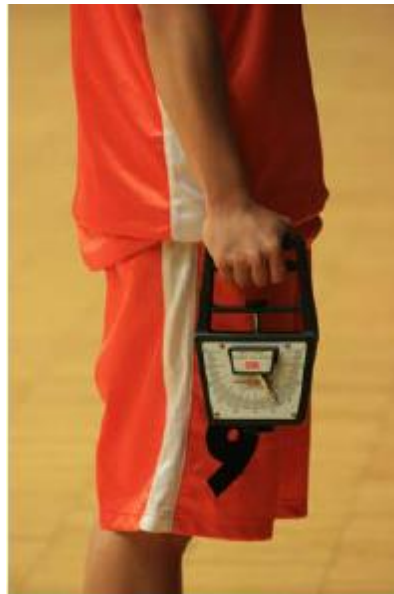
Fig. 4.8 Measuring muscular strength with a handgrip dynamometer
