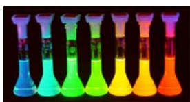
Fluorescence of CdSe QD under UV exposure
