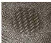
High resolution transmission electron micrograph of CdSe (adapted from www.people.man.ac.uk/~mbdsspo2/nanodis.html )
