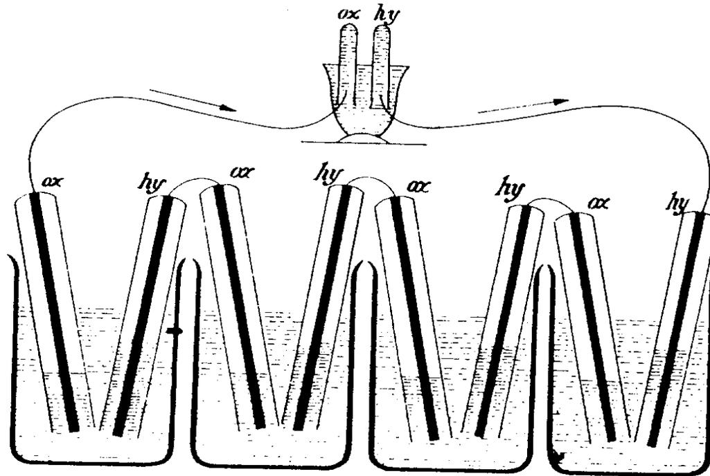
Fig. 1.5 *Four cells of Groves H<sub>2</sub>/O<sub>2</sub> battery, used, in Grove's words, 'to effect the decomposition of water by means of its composition'*
