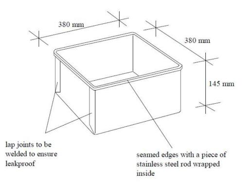
Overall dimension 380 mm x 380 mm x 145 mm, to be made of a SWG 24 stainless steel (type 316) sheet. All edges should be seamed with a piece of stainless steel rod (diameter 5 mm) to stiffen and avoid sharp edges. The lap joints should be welded to ensure that the whole tray is leak-proof.
