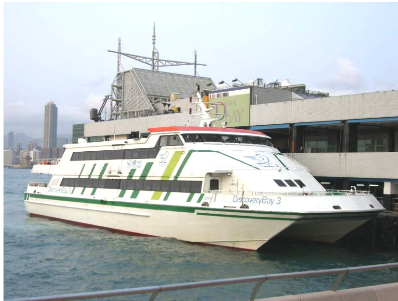
(2) Boat hull made of GRP
