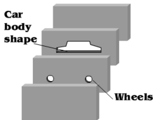
Exploded view of a laminated mould
