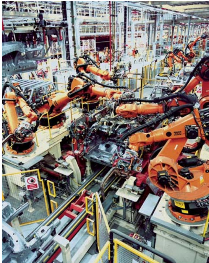
Figure 3.18 Work cells in FMS / car production
