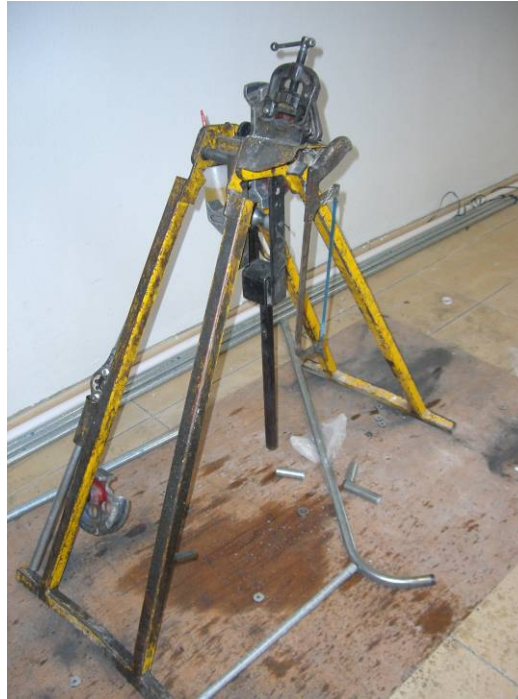
Figure 2.16 Hand-operated bending tool with circular face and roller control
