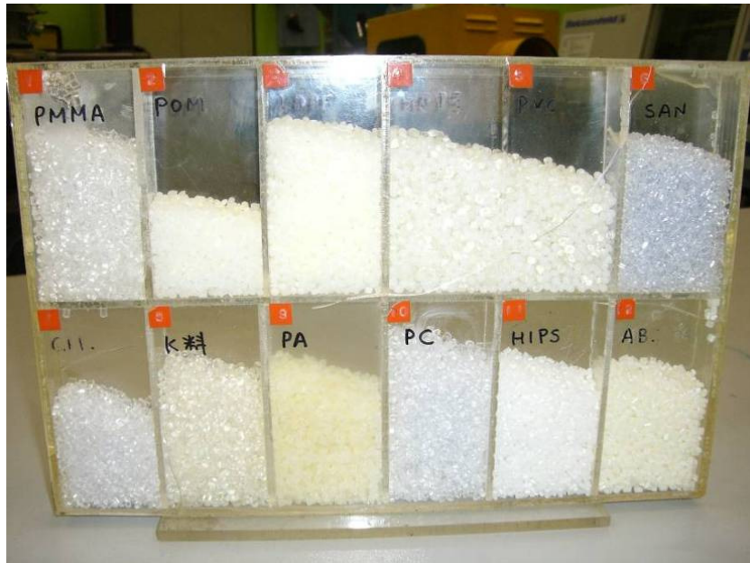
Figure 2.10a Different plastic beans used for injection moulding
