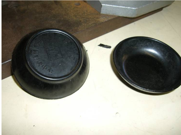
Figure 2.35 Compression moulded dishes
