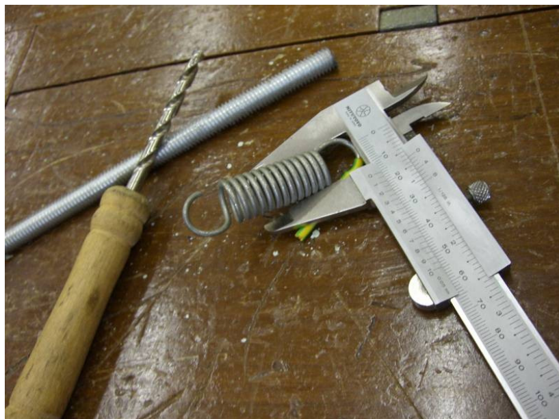
Figure 2.64 Using caliper makes a precise measurement
