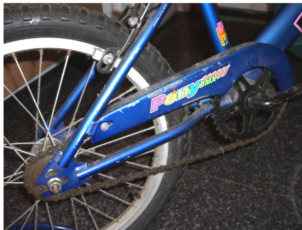
Figure 1.41 Chain drive of a bicycle
