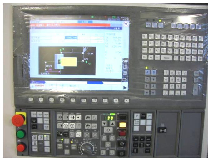
Figure 3.3 Computer screen simulation of the cutting process
