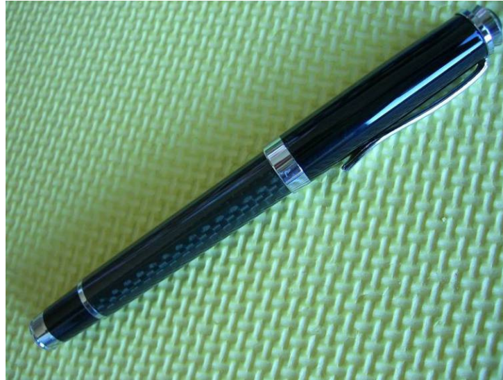
Figure 1.47 Pen barrel made of carbon fibre reinforced plastic
