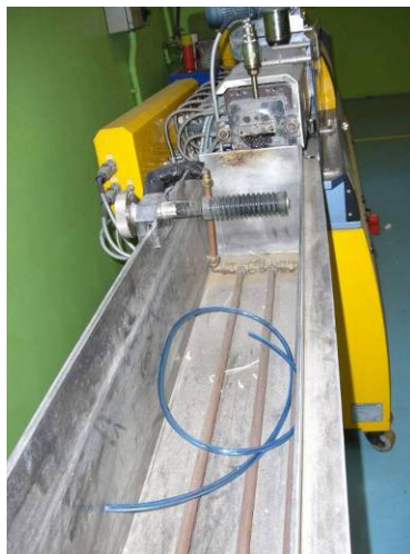
Figure 2.41 Water bath for cooling
