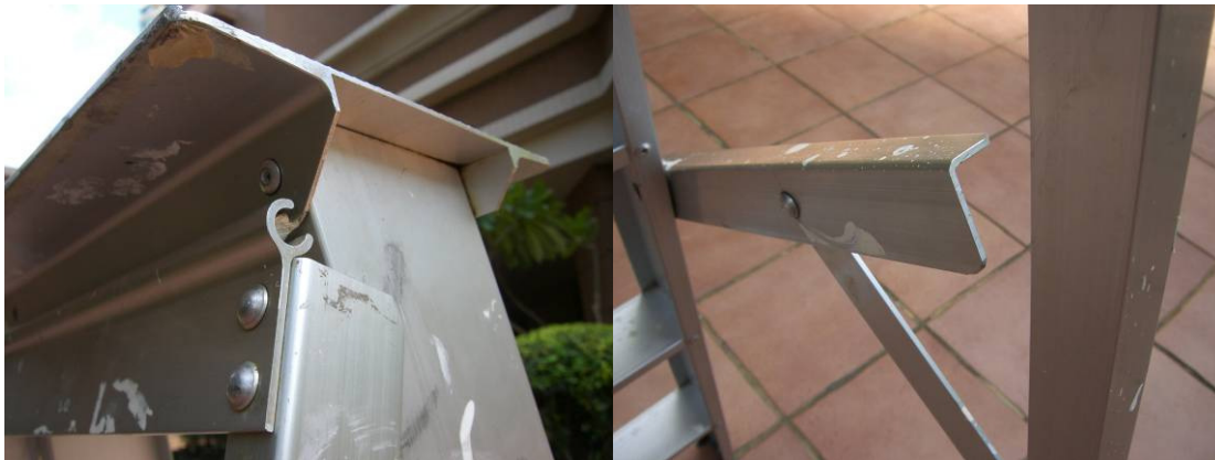
Figure 2.42 Cross-sections of shapes that are easily being extruded.
