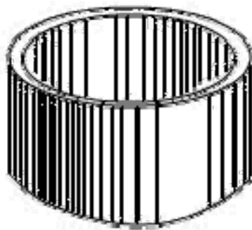
Low line density shows the light surface of a cylinder
