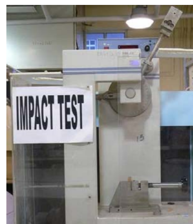
Impact testing machine
